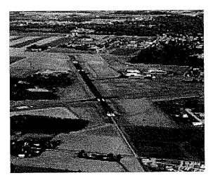
The crosswind runway (04/22) is 3,600 feet in length with a width of 100 feet and is constructed of bituminous concrete. Lighting aids on this runway include MIRLs and REILs on Runway 04. Instrument approaches to the airport include a Simplified Directional Facility to Runway 34, Non-directional Radio Beacon approach to Runway 04 and 16 and a Very High Frequency Omnidirectional Radio Range.
